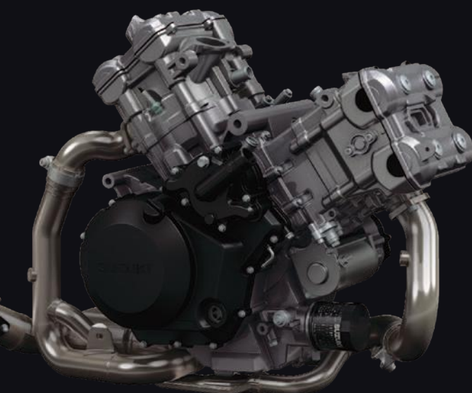
1037cm 3 DOHC, 90-degree V-twin engine
